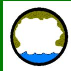
The start of a blocked pipe begins when grease and solids collect on the top and sides of the pipe interior.
